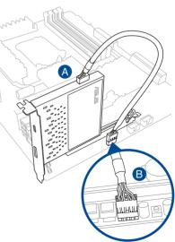
Connect the DisplayPort cable to the ThunderboltEX II card's DisplayPort IN port (A) and to the DisplayPort or mini DisplayPort on the motherboard's I/O port (B).
