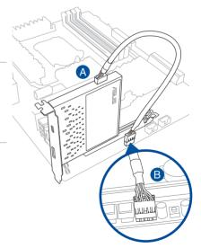
For supported 9 Series motherboards, use the bundled TB\_Header converter to connect your ThunderboltEX II card to the TB\_Header port on the motherboard.
