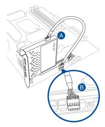
Connect the DisplayPort cable and the mini DisplayPort cable to the ThunderboltEX II/DUAL card's DisplayPort IN ports (A) to the DisplayPort (B) and the mini DisplayPort (C) on the motherboard's I/O port.
