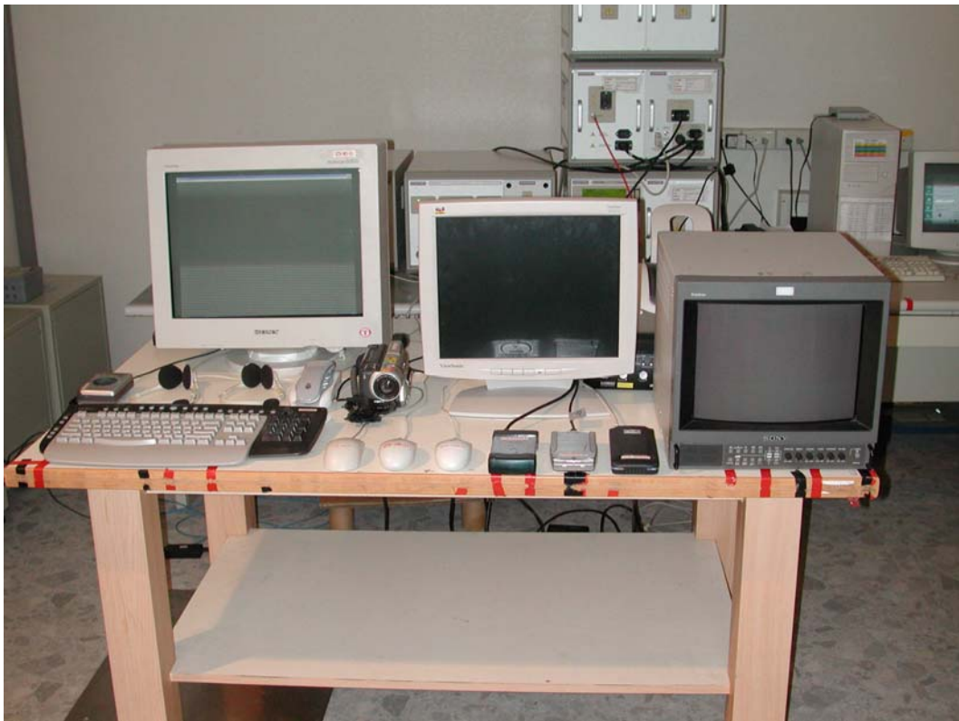
Voltage Dips Test Setup (Mode 1)
