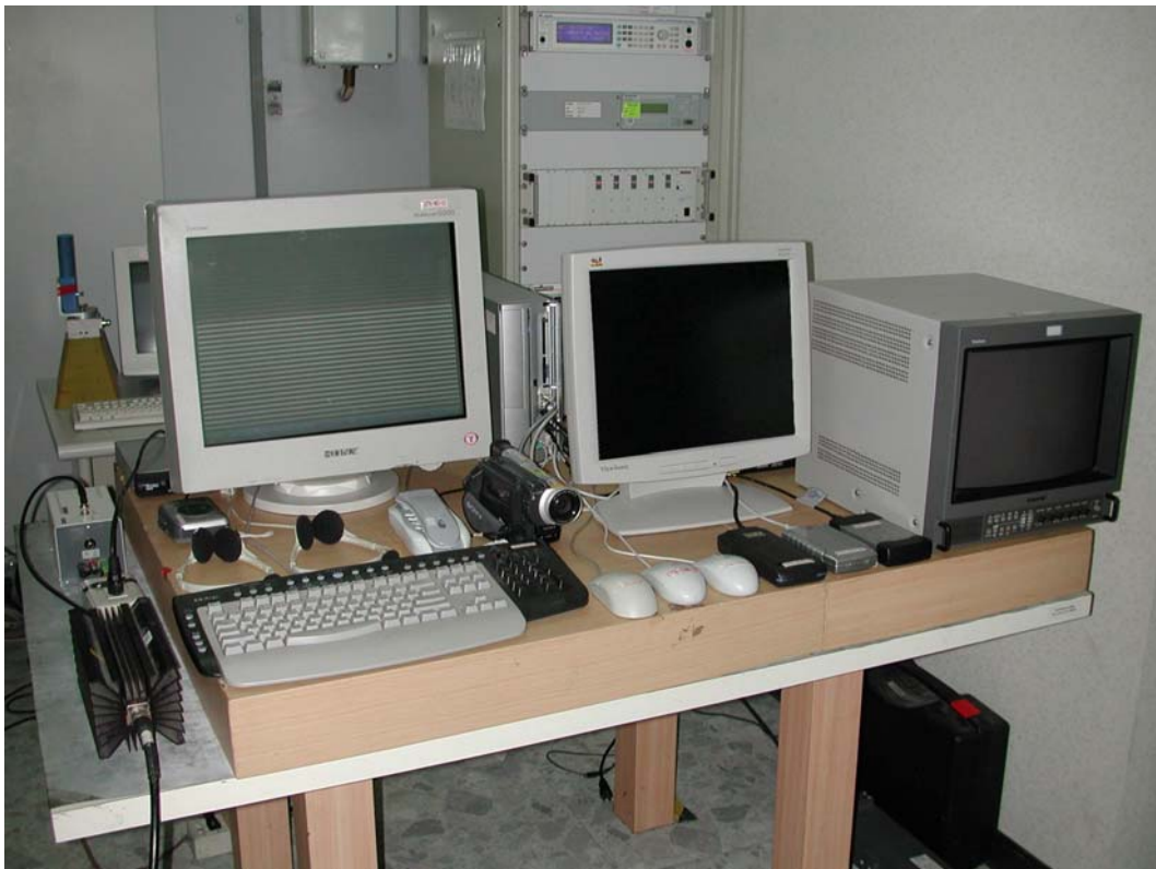
Conducted Susceptibility Test Setup (Mode 1)
