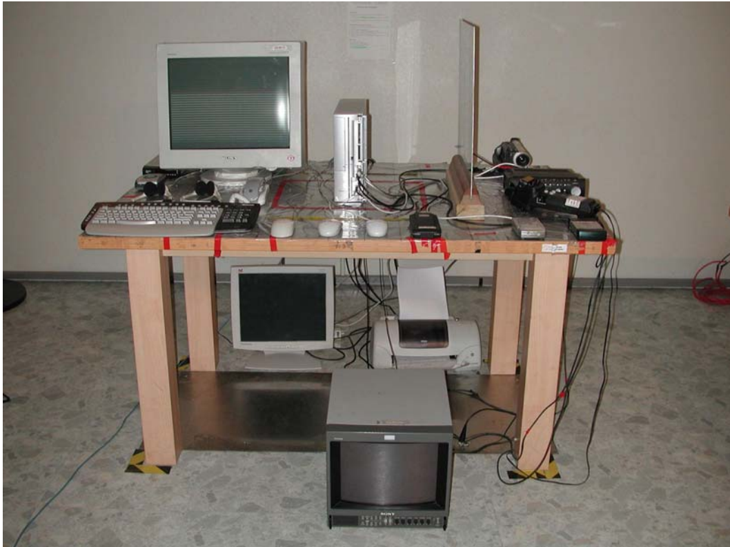
ESD Test Setup (Mode 1)
