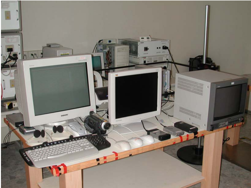
Power Frequency Magnetic Field Test Setup (Mode 1)
