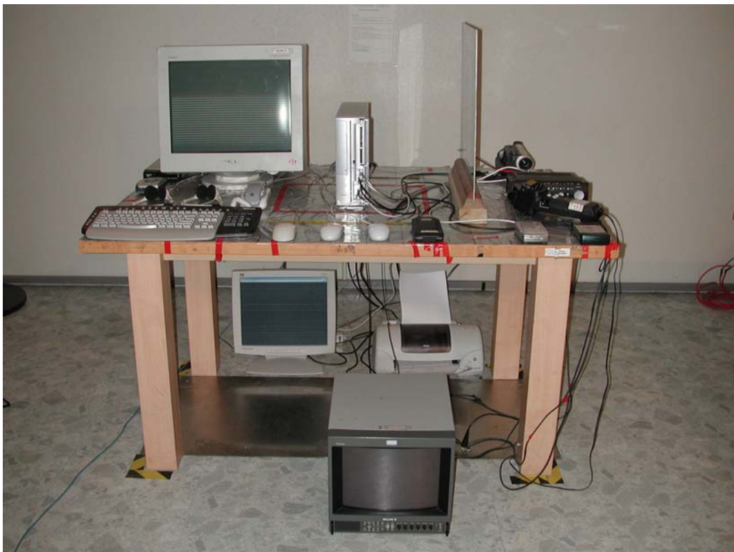
ESD Test Setup (Mode 2)
