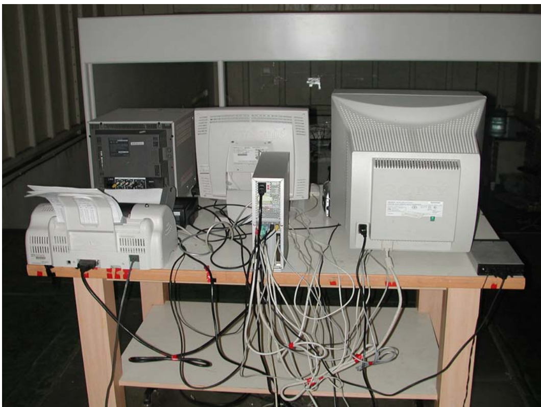
Back View of Radiated Test (Mode 1)
