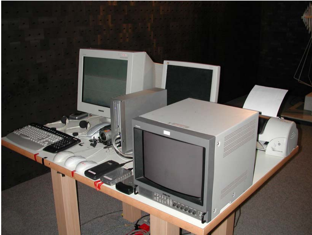
Radiated Susceptibility Test Setup (Mode 1)
