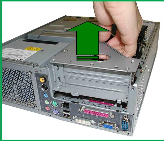
1. To remove the I/O cover from the chassis, pull-out the expansion card assembly.
