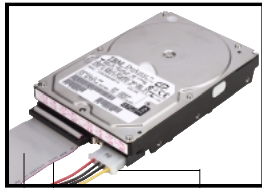
Red Stripe to Pin 1 IDE Ribbon Cable Power Cable (P3)
