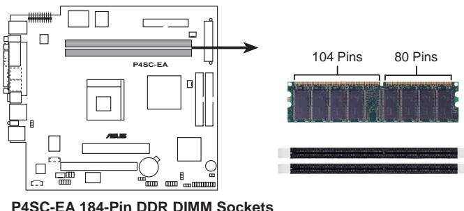
P4SC-EA 184-Pin DDR DIMM Sockets
