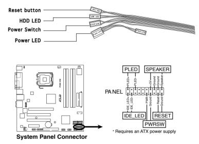
Connect the **reset button**, **power switch**, **power LED**, and **HDD LED** cables to their respective leads in the system panel connector on the motherboard. See page 4-11 for the system panel descriptions.
