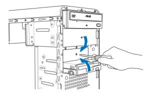
3. With the HDD label side up, carefully insert the drive into the 3.5-inch bay and push the drive into the bay until its screw holes align with the holes on the drive bay.
