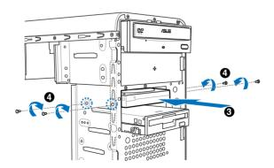
4. Secure the drive with two screws on both sides.
