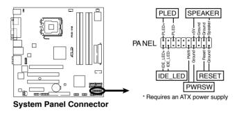
The sytem panel connector is color-coded for easy connection. Refer to the connector description below for details.
