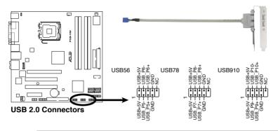
Never connect a **1394 cable** to the USB connectors. Doing so will damage the motherboard!
