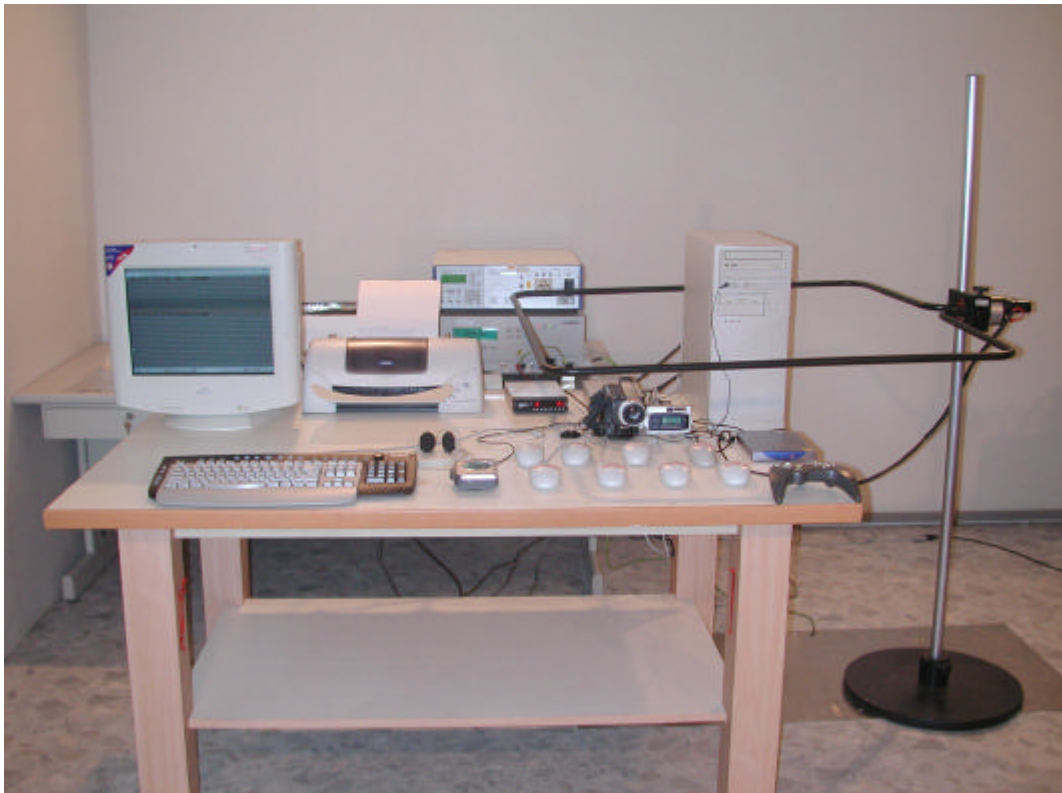
Power Frequency Magnetic Field Test Setup
