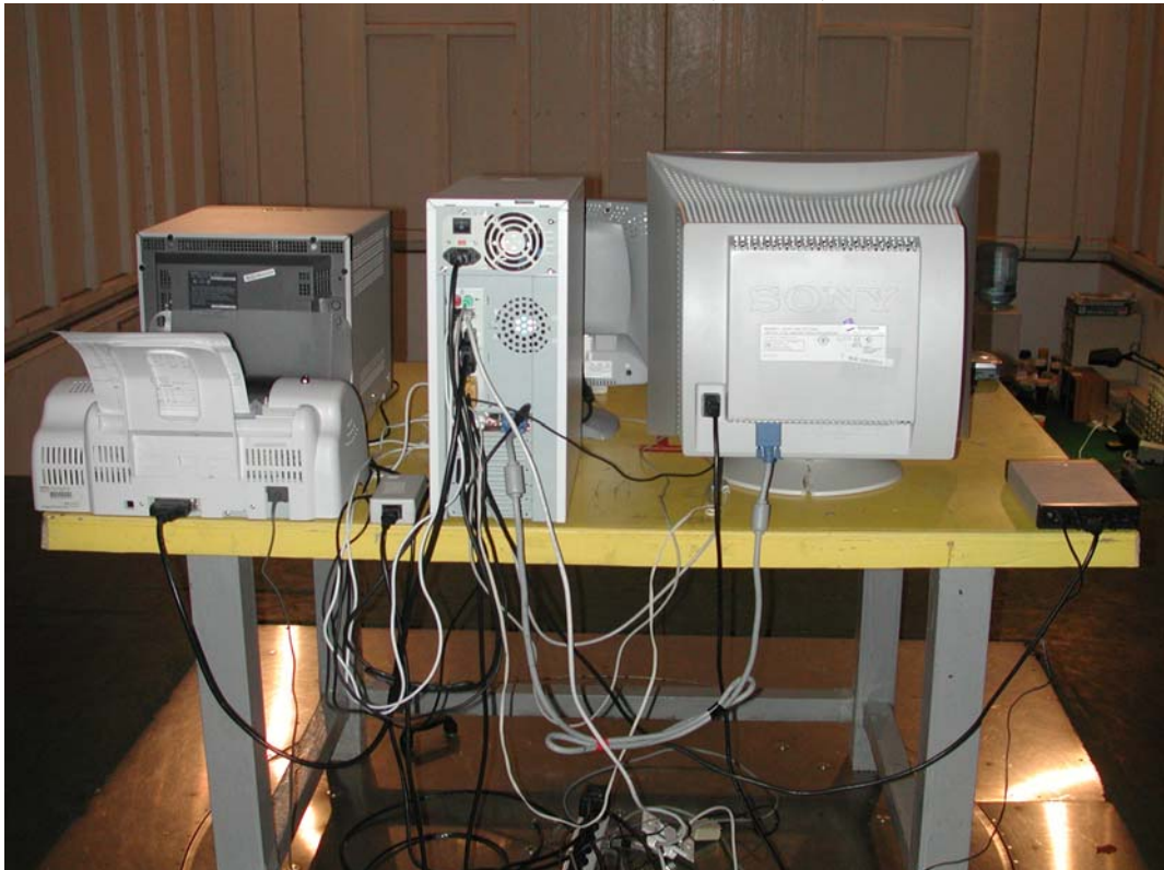
Back View of Radiated Test (Mode 2 )
