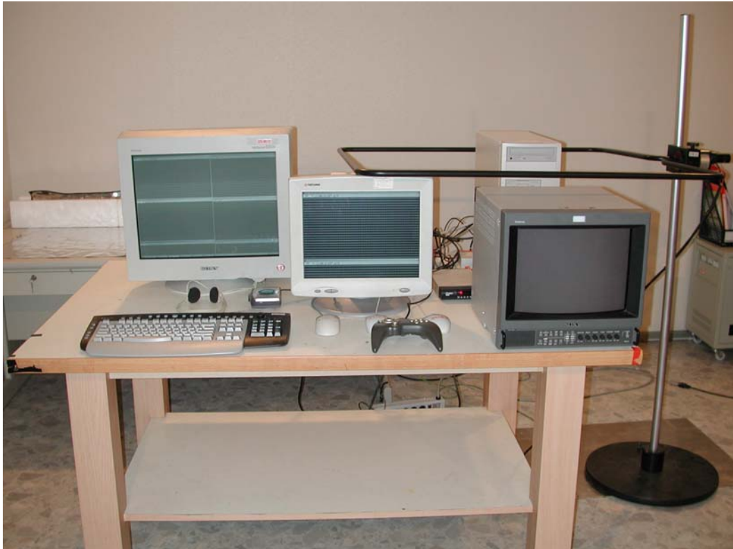
Power Frequency Magnetic Field Test Setup
