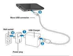
CAUTION! Double-check the connections and ensure that the power plug is securely attached to the AC Adapter to prevent overheating and damage to the cables, adapter, or device.
