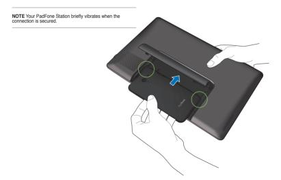
4. Close the PadFone bay door and ensure that the latch firmly locks in place.
