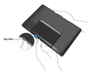
Push the PadFone bay door up to a ninety-degree (90°) angle until the PadFone detaches completely from the connectors.
