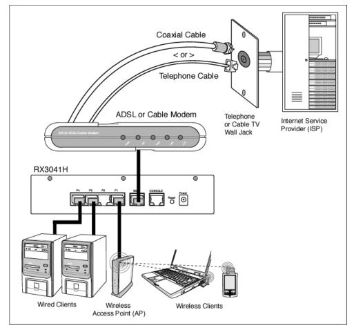
Figure 3.1. Overview of Hardware Connections
