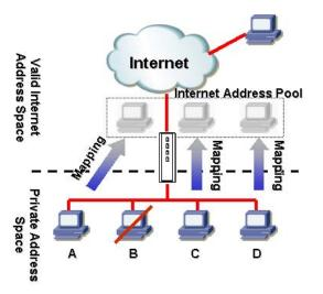
Figure 9.3 Dynamic NAT – PC-A can get an NAT association after PC-B is disconnected
