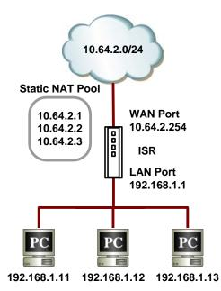
Figure 9.31. Network Diagram for NAT Pool Example
