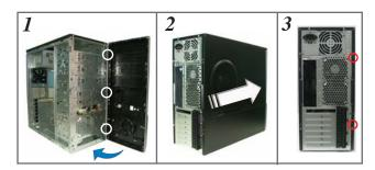
Push the bay lock upward. Insert the HDD into the bay. Align the HDD holes with the bay holes, then push down the bay lock to secure the HDD. the HDD.
