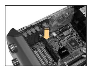
6. Secure the card with the lock tab you removed earlier.
