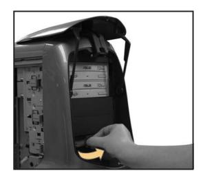
3. Using a screwdriver, push the knock down metal cover in and out of the chassis until it is removed.
