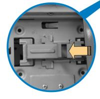
4. Carefully insert the optical drive into the bay, then push it inward until it is completely flushed to the chassis front panel.
