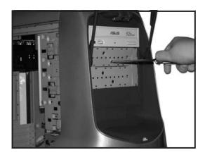
4. Slide the drive bay lock to the left, towards the ♂ sign, to unlock the drive bay.
