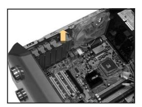
5. Align the card connector with the slot, then press firmly until the card is completely seated on the slot.
