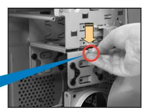
2. Carefully pull the cage out of the chassis in the direction of the arrow. Place the HDD cage on a flat surface.
