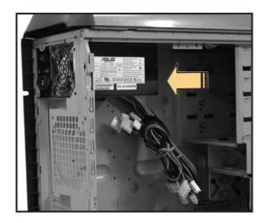
3. Secure the PSU with screws.
