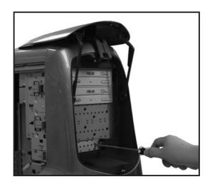
3. Slide the drive bay lock to the right, towards the ♂ sign to unlock the drive bay.
