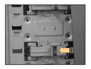
5. Carefully insert the optical drive into the bay, then push it inward until it is completely flushed to the chassis front panel.
