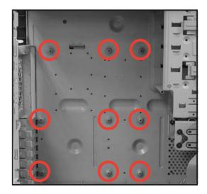
3. Orient the motherboard such that its screw holes match with the mounting plate holes on the chassis.
