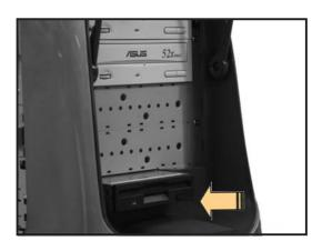
5. Slide the drive bay lock to the left, towards the  $\bigcirc$  sign to lock the drive bay and to secure the drive in place.
