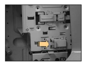
4. Carefully insert the floppy disk drive into the bay, then push it inward until it is completely flushed to the chassis front panel.
