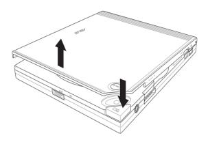
2. When the top cover opens, carefully lift the top cover fully upward.
