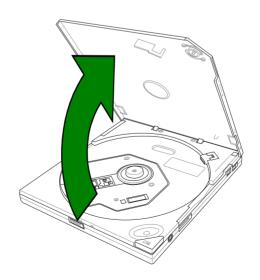
3. Place the disc into the tray and make sure the disc is securely clipped in place.
