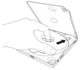
4. Close the top cover by gently pressing the cover downwards until the top cover locks in place.
