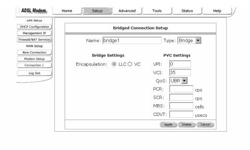
Figure 4 (Bridge Connection Setup)
