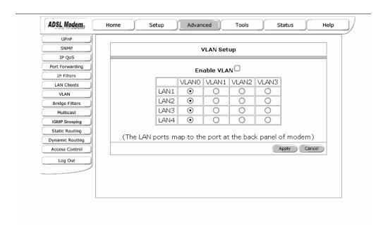
Figure 19 (VLAN Setup)
