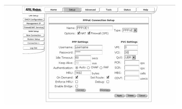
Figure 6 (PPPOE Connection Setup)
