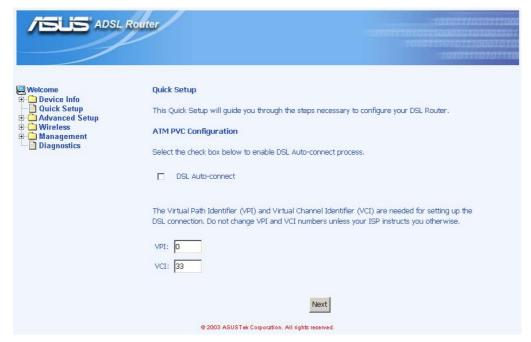
Figure 5.1 DSL Auto-connect or Manually VPI/VCI input
