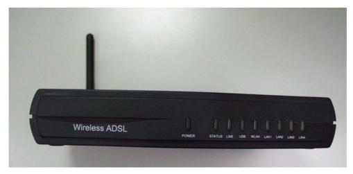
Figure 2.2 Front Panel LEDs
