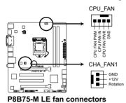
Do not forget to connect the fan cables to the fan connectors. Insufficient air flow inside the system may damage the motherboard components. These are not jumpers! Do not place jumper caps on the fan connectors!
