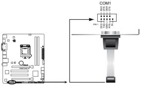
P8B75-M LE Serial port (COM1) connector
