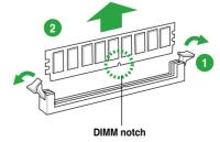
2. Remove the DIMM from the socket.
