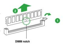
2 Remove the DIMM from the socket
