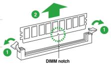
2. Remove the DIMM from the socket.
