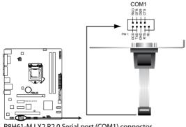
P8H61-M LX2 R2.0 Serial port (COM1) connector
