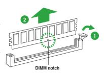
2 Remove the DIMM from the socket
