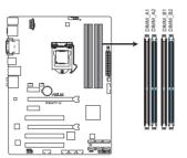
P8H77-V 240-pin DDR3 DIMM sockets
