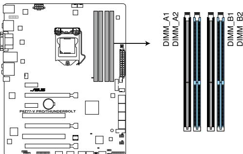
P8Z77-V PRO/THUNDERBOLT 240-pin DDR3 DIMM socket
