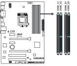
Z77-A 240-pin DDR3 DIMM sockets
