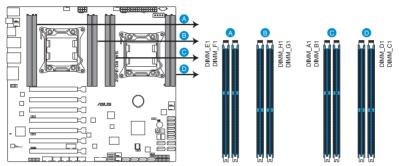
Z9PE-D8 WS 240-pin DDR3 DIMM sockets
