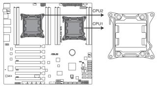
Z9PE-D8 WS CPU LGA2011 Socket
