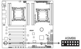
**Z9PE-D8 WS ASMB connector**
