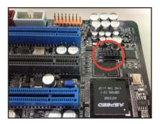
2. Orient and press the ASMB6 management card in place
