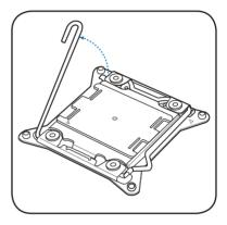
4. Press the right load lever with your thumb (C), then move it to the right (D) until it is released from the retention tab. Lift the load lever in the direction of the arrow (E).
