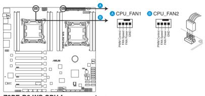
**Z9PE-D8 WS CPU fan connectors**
