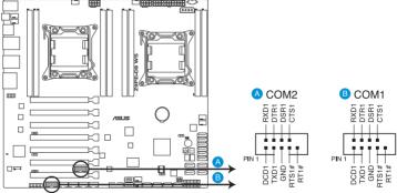
Z9PE-D8 WS Serial port connectors
