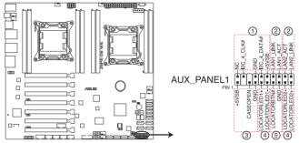
**Z9PE-D8 WS Auxiliary panel connector**
