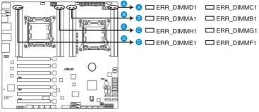
**Z9PE-D8 WS ERR DIMM LED**
