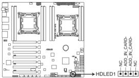
Z9PE-D8 WS Hard disk activity LED connector
