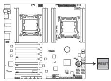
**Z9PE-D8 WS Reset switch**
