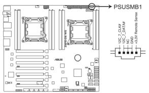
**Z9PE-D8 WS Power supply SMBus connector**
