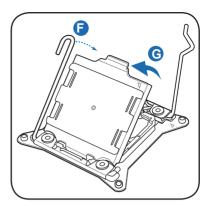
Position the CPU over the socket, ensuring that the triangle mark is on the top-right corner of the socket.
