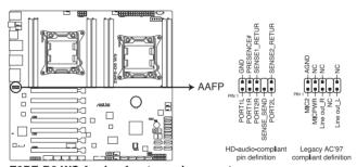
Z9PE-D8 WS Analog front panel connector
