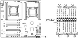
Z9PE-D8 WS System panel connector
