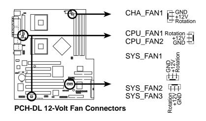
Do not forget to connect the fan cables to the fan connectors. Lack of sufficient air flow within the system may damage the motherboard components. These are not jumpers! DO NOT place jumper caps on the fan connectors!
