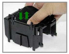
8. Align the two pegs on the air tunnel with the corner holes of the fan module. Press the module down until the four hooks on the air tunnel snap on its sides.
