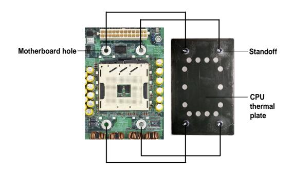
2. Place the heatsink retention mechanism over the CPU socket, matching its holes with the four holes on the motherboard and the standoffs on the thermal plate.
