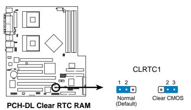
Except when clearing the RTC RAM, never remove the cap on CLRTC jumper default position. Removing the cap will cause system boot failure!
