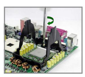
4. Position the heatsink on top of the CPU, having its angled side (with cut corners) facing the memory sockets. Make sure that the heatsink base fits completely on the retention mechanism.
