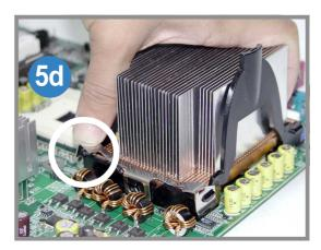
6. Follow step 5 to install the other retention clip, and completely secure the heatsink.
