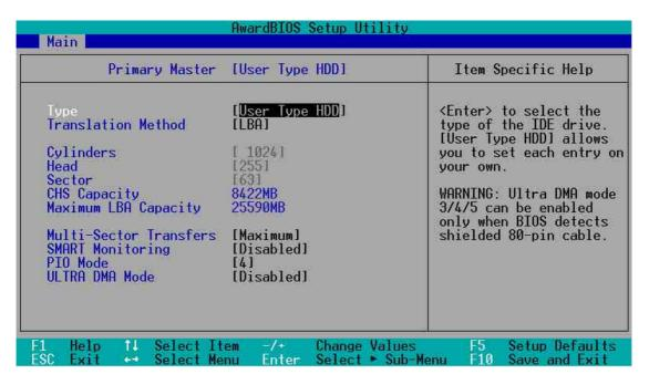
Manually enter the number of cylinders, heads and sectors per track for the drive. Refer to the drive documentation or on the drive label for this information.
