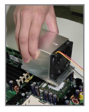
2. Hook one end of the retention bracket into the protruding tab on the corner of the plastic retention base. (The retention base comes installed with the motherboard.)
