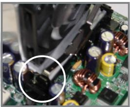
Use a small flat screw driver to attach the other end of the bracket, while firmly holding down the heatsink and fan assembly. The middle hook of the bracket snaps in place if you properly attached the two ends.
