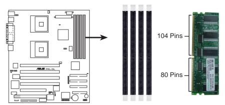
PRL-DL 184-Pin DDR DIMM Sockets
