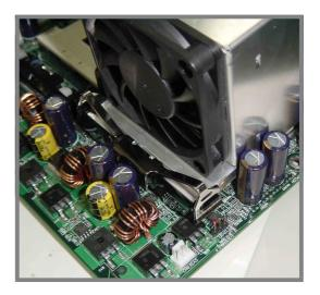
6. When the heatsink and fan assembly is in place, connect the fan cable to the fan connector on the motherboard labeled FAN1 (for the CPU on socket 1) and FAN2 (for the CPU on socket 2).
