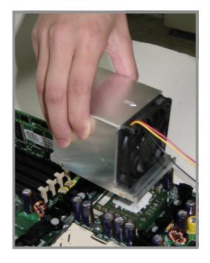
2. Hook one end of the retention bracket into the protruding tab on the corner of the plastic retention base. (The retention base comes installed with the motherboard.)
