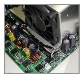
6. When the heatsink and fan assembly is in place, connect the fan cable to the fan connector on the motherboard labeled CPUFAN1 (for the CPU on socket 1) and CPUFAN2 (for the CPU on socket 2).
