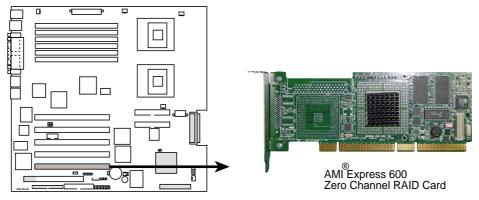
**PR-DLS Zero Channel RAID Slot**
