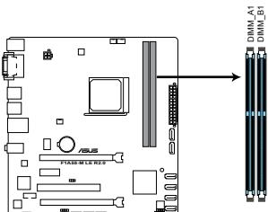
**F1A55-M LE R2.0 240-pin DDR3 DIMM sockets**
