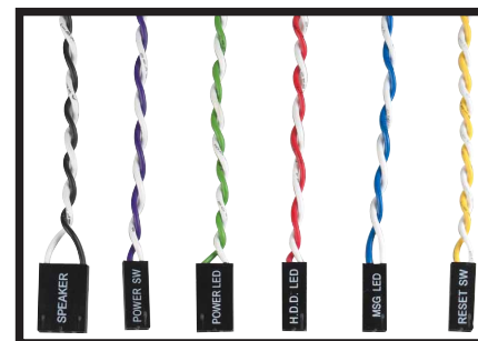
LED and switch leads
