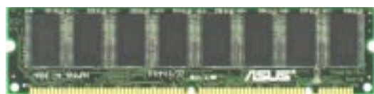
SDRAM DIMM (8 chips, Non-ECC)
