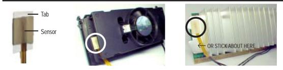
**WARNING!** Do not insert the sensor between the processor and heatsink, otherwise, it will cause damage to the P2T-Cable.
