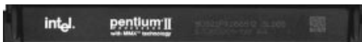
Intel Pentium II Processor in an SEC cartridge (233-450MHz 512KB/128KB/0KB L2 Cache)
