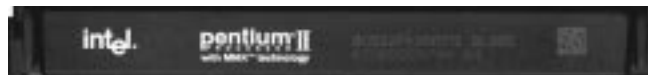
Intel Pentium II Processor in an SEC cartridge (233-450MHz 512KB/128KB/0KB L2 Cache) CPU (Item 9)
