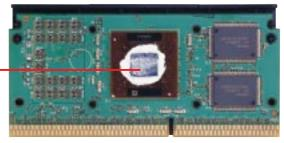
The thermal interface material should be continuous with no through-holes or debris.
