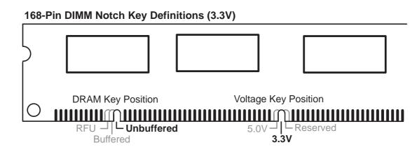
The notches on the DIMM will shift between left, center, or right to identify the type and also to prevent the wrong type from being inserted into the DIMM slot on the motherboard. You must tell your retailer the correct DIMM type before purchasing. This motherboard supports four clock signals per DIMM. 3. H/W SETUP System Memory
