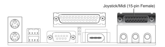
8) Audio Port Connectors (Three 1/8" Female) (with optional onboard audio)
