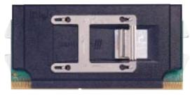
Example of an incorrectly installed retention clip
