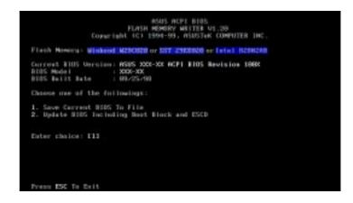
**IMPORTANT!** If "unknown" is displayed after **Flash Memory:**, the memory chip is either not programmable or is not supported by the ACPI BIOS and therefore, cannot be programmed by the Flash Memory Writer utility.
