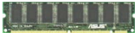
Non-ECC SDRAM DIMM (8 chips)
