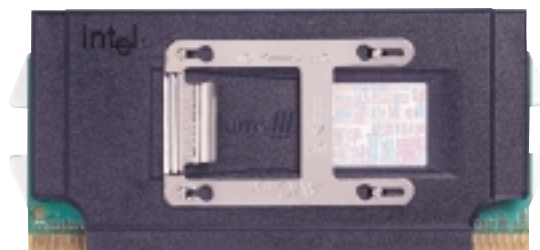
Example of an incorrectly installed retention clip
