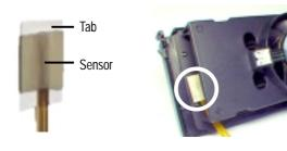
**WARNING!** Do not insert the sensor between the processor and heatsink, otherwise, it will cause damage to the P2T-Cable.
