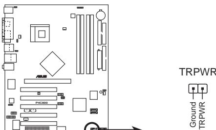
P4C800 Power Supply Thermal Connector
