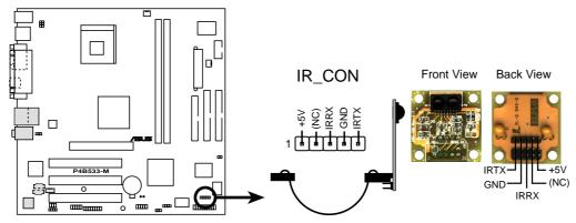
P4B533-M Infrared Module Connector
