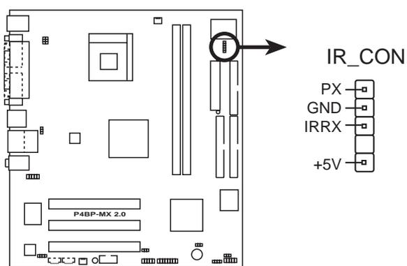
**P4BP-MX 2.0 Infrared Module Connector**
