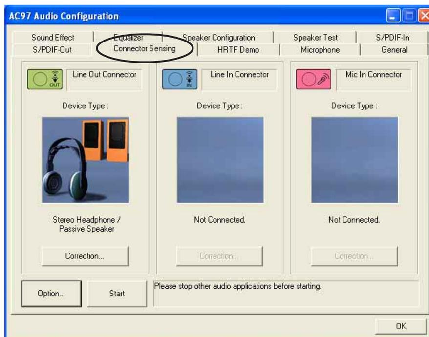
The Realtek® EZ-connection dialog box shows your current audio connections. The text at the bottom of the box explains your audio connection status. An *X mark* denotes an incorrect connection.
