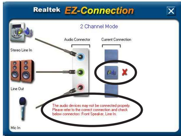
If there are detected problems, make sure that your audio cables are connected to the proper audio jack and repeat connector sensing.
