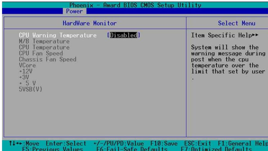
The items in the Hardware Monitor sub-menu displays the status of the hardware devices monitored by the system.
