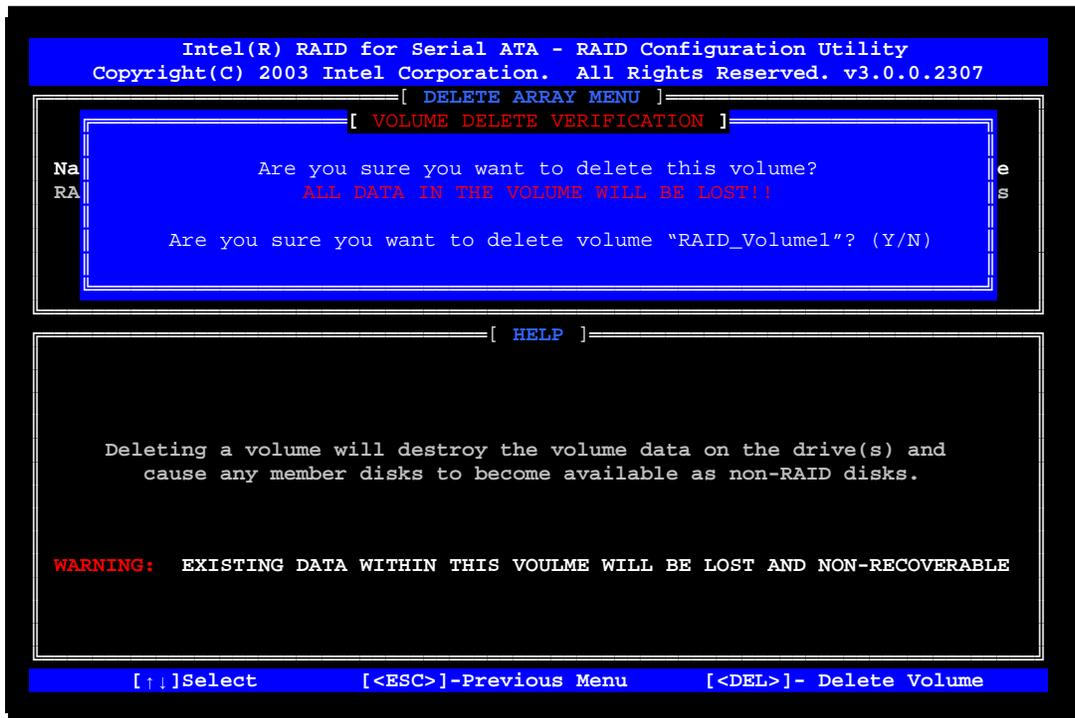
3. Confirm the volume deletion by pressing the <Y> key.
