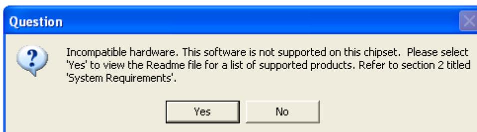
*Resolution:* This issue is resolved by installing the Intel Application Accelerator RAID Edition on a system with a [supported Intel chipset](#).
