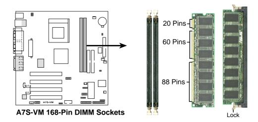
The DIMMs must be 3.3Volt unbuffered SDRAMs. To determine the DIMM type, check the notches on the DIMMs (see the figure below).
