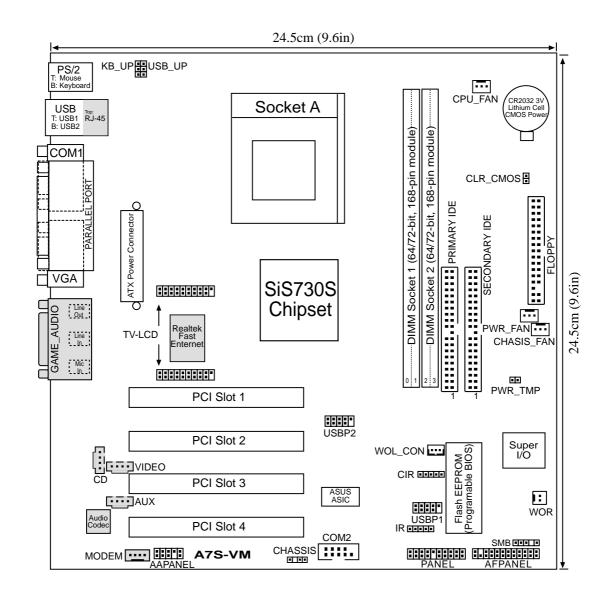
**NOTE:** The Audio Codec, external and internal audio connectors, RealTek RTL8100 chipset, and RJ-45 LAN connector are optional components. These items are grayed out in the above motherboard layout.
