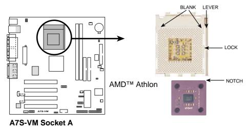
Note in the illustration that CPUs have marks (usually a notch or a gold mark on one corner) to help you identify the proper orientation and enable you to correctly install a CPU. It is important that you match the marked corner of the CPU with the corresponding corner on the socket so as not to damage the CPU pins.
