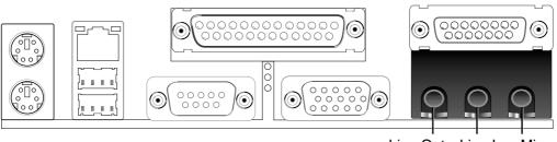
Line Out Line In Mic 1/8" Stereo Audio Connectors
