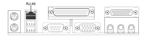
4) Universal Serial BUS Ports 1 & 2 (Black two 4-pin USB) Two USB ports are available for connecting USB devices.
