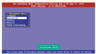
The screen displays the available RAID set(s) and prompts you to select the virtual drive to initialize. Use the arrow keys to select the virtual drive from the Virtual Drive selection, and then press <Space>.
