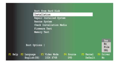
Insert the RAID driver disk to the floppy disk drive. Type the command acpi=off apic=bigsmp brokenmodules=ahci in Boot Options field, and press <Enter>.
