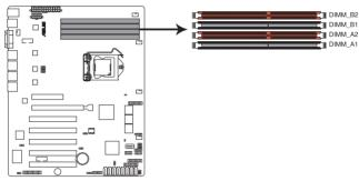
P8B-C Series 240-pin DDR3 DIMM sockets
