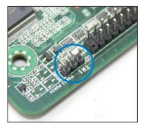
2. Connect the thermal sensor cable to the connector.
