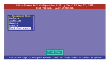
The screen displays the available RAID set(s) and prompts you to select the virtual drive to check. Press <Space> to select the virtual drive from the Virtual Drive sub-menu, and then press <F10>.
