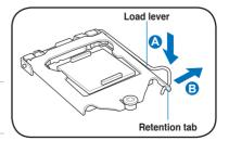
3. Lift the load lever in the direction of the arrow until the load plate is completely lifted.
