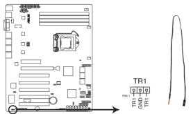
P8B-C Series Thermal sensor cable connector
