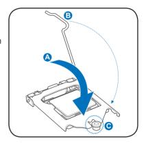
8. Insert the load lever under the retention tab.
