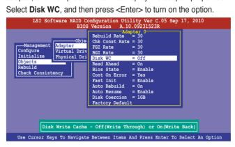
3. From the **Management Menu**, select **Objects** > **Virtual Drive**, select an existing adapter and press <Enter>. Select View/Update Parameters and press <Enter> to display the adapter properties.
