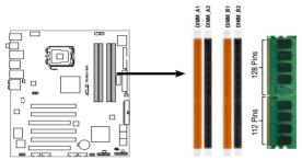
P5K64 WS 240-pin DDR3 DIMM Sockets
