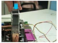
Carefully push down the fan until it snugly fits the heatsink, then connect the fan cables.
