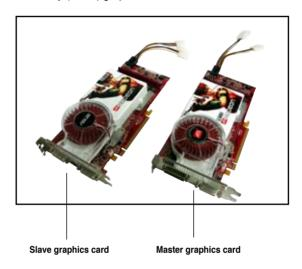
Insert the CrossFire™ Edition (Master) graphics card into the PCI Express x16 <u>blue</u> slot. Make sure that the card is properly seated on the slot.
