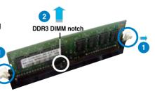
Remove the DIMM from the socket.
