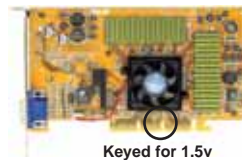
P5VDC-MX Accelerated Graphics Port (AGP)
