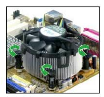
Pull up two fasteners at a time in a diagonal sequence to disengage the heatsink and fan assembly from the motherboard.
