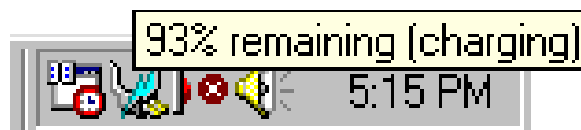
Power icon using AC power. The charging (lightning) icon appears over the “plug” icon if the battery is not fully charged. When fully charged, only the “plug” icon will remain.
