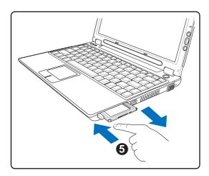
2. Press the extended button again to eject the PC Card. Carefully pull the ejected PC card out of the socket.
