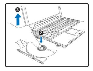
2. While pressing down on the center hub, gently pry the edge of the disc upwards at an angle to remove the disc from the hub.
