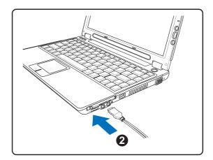
3. Carefully connect any cables or adapters needed by the PC card. Usually connectors can only be inserted in one orientation. Look for a sticker, icon, or marking on one side of the connector representing the top side.
