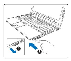
1. Press in the toggle eject button and release. The recessed spring loaded toggle button will extend when pushed in and released.
