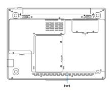
TIP: Use a straightened paper clip to press the shutdown button.
