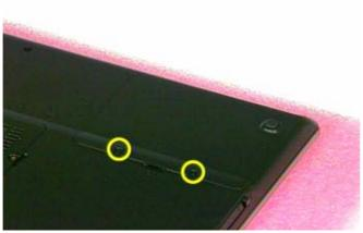
3. Pull up the HDD module a little bit and disconnect the HDD
