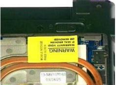
Note: If fan module has no thermal pad on it, please plus a thermal pad on the CPU die before assembling.
