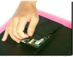
2. If there is an existing memory, remove it by opening the latches, which will pop the module up to a 45° angles, and then pulling out the module in that angle.
