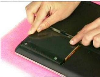
6. Secure 2 screws on the bottom to affix the HDD module.
