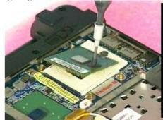
2. Turn the non-removable screw here 180 degrees clockwise to fix the CPU and stick thermal pad on the CPU die
